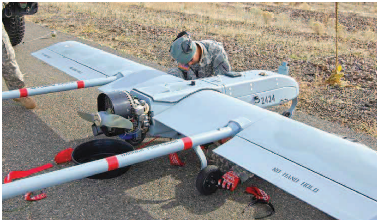
ALL SYSTEMS GO A 1st SFG(A) Tactical Unmanned Aerial Vehicle Systems Soldier conducts a preflight inspection of the RQ-7B Shadow. U.S. Army photo by SFC Charles Gaither.
